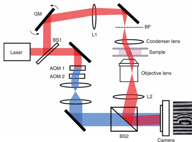
**Figure 1** | Tomographic phase microscope. BS1 and BS2, beamsplitters 1 and 2; GM, galvanometer scanning mirror; L1, focal length  $f = 250$ -mm lens; BF, back focal plane of condenser lens; L2,  $f = 200$ -mm lens. The sample laser beam with original laser frequency is shown in red, and the frequency-shifted reference laser beam is shown in blue. A typical fringe pattern for a tilted beam illuminating a single HeLa cell is shown.
