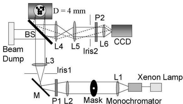
Fig. 2.  $\phi$ /LSS experimental system. BS, beam splitter; M, mirror. Other abbreviations defined in text.
